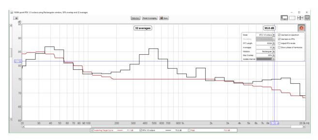
Now, we've about as close as we're going to get to the target curve using just the level controls for the individual channels and we'll use our equalizer to finish the job.
