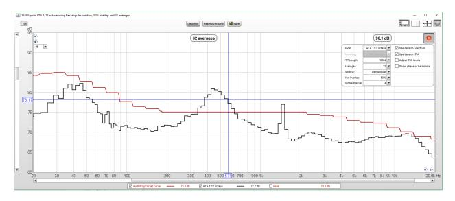
Bandwidth is the higher frequency at which the level is down by 3 dB minus the lower frequency. In this case,
