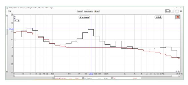
if you click on the display at the top of the peak, REW will display a cross hatch and in the blue boxes, the program will tell you the frequency and the level. So, in the example above, we can see that the peak in our response is about 500 Hz. We can also see that the level of the peak is 11.6dB higher than our target level of 75 dB. So, in our text entry box for our filter, we can enter 500 H for the frequency and -11.6 dB for the amount of cut.
