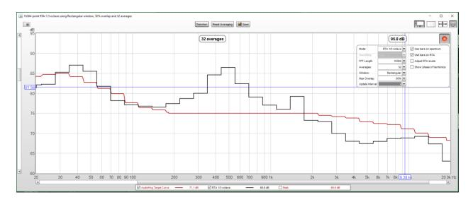
Above 2 kHz, we don't have enough tweeter level. We'll turn up the level of the tweeter channel on this side by about 6 dB to get closer to the target curve.
