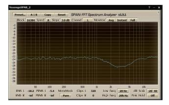
So, our RTA shows us a dip in the response and we "fix" it by adjusting the crossover points or by using the EQ. If we use the EQ to boost a bit so the response is closer to our target curve, this is what the RTA will show us:
