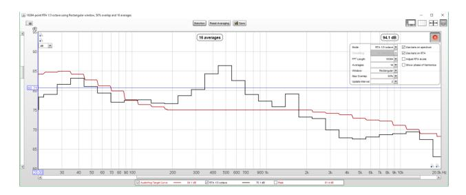
In the 3-way front speaker system we're going to optimize in this example, the crossover between the midrange and the tweeter is 2.2 kHz. The crossover between the midrange and the midbass is 300 Hz. The high pass filter for the midbass is 80 Hz and the subwoofer low pass filter is at 60 Hz. The delays have been set using the tape measure and all of the electrical polarity has been confirmed.
