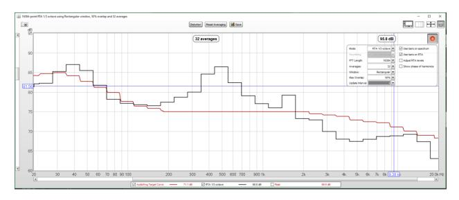
Moving to the right, and thinking about the level of the midrange, we can see that at between 300 Hz and 2 kHz, we have a couple of big peaks to remove, but at the base of the big peaks, the level is about right. We'll leave the midrange level control alone.
