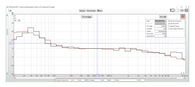
Finally, another filter at about 15 kHz, a cut of -4 dB and a Q of 1.4 should do it.
