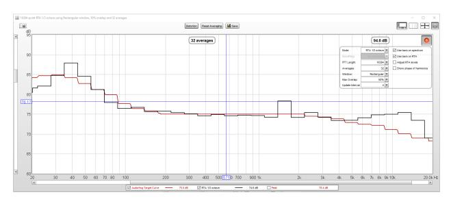
Next, we can apply a single band at 1.6 kHz to get rid of that peak. We know that the Q of this filter should be high, so we'll try 10.
