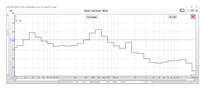
Notice that at the bottom, there's a check box to display the active measurement and also a check box for the target curve to the left. Adjust the resolution of the RTA window to show 5dB per division using the "+" and "-" buttons and be sure that "dB" rather than dBFS" is chosen in the top left corner. Use the scroll bar on the left to center your measurement in the display.
