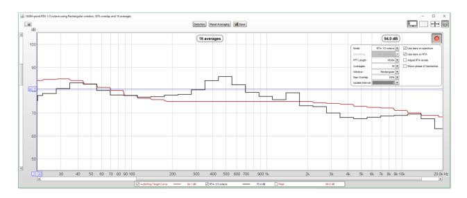
If the horizontal scale at the bottom isn't 20Hz-20kHz, click on the Graph Limits button next to the wheel and set the limits by typing into the boxes.
