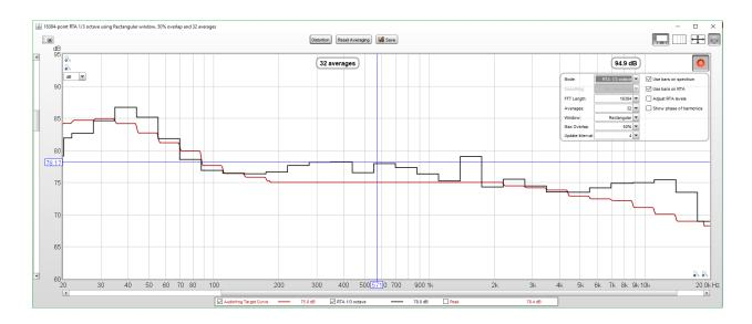
That gets us pretty close. Now we can just adjust the level and the Q a little bit. I've changed the level to -12 dB and the Q to 1.9 to arrive at the result below.
