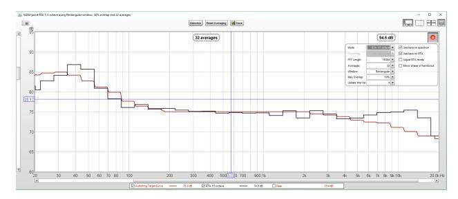
Now, that peak is gone. Let's work on the high frequencies a bit. Let's try a filter at 10 kHz, acut of 4.5 dB and a Q of 1.4.
