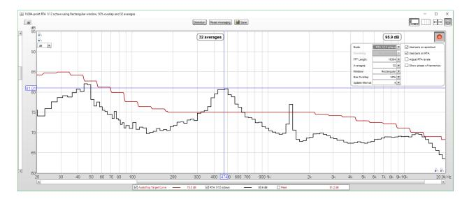
Now, we can see the peak a little more clearly. Move the cursor to the center frequency if it now appears slightly to the left of to the right. I've moved it to 474 Hz. Notice that the level at that peak is 81 dB. We're looking for the point to the left and to the right at which the level is 3 dB lower—78 dB. Move you're the cursor to the left until you see 78dB and read the frequency. In this case, it's 398 Hz.
