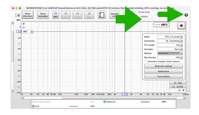
**Step 6**. To start the RTA, click on the red "record" button. Start Track 1 on the Tuning CD and measure the frequency response of the system.
