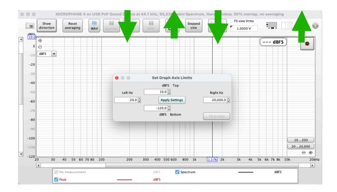
**Step 5**. Click on the "Settings" wheel and in the top drop down box, choose 1/3 Octave fir the Mode. Choose 32768 for the FFT length. Choose None for Averages. Choose "Rectangular" for the Window. Choose 50% for Max Overlap. Select "Bars" for the RTA and for "Spectrum". Click the settings wheel to close the box.
