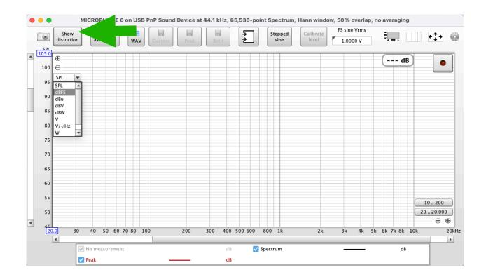
**Step 4**. Click on the "Limits" box at the top right of the display and enter "20" in the Left box and 20000 in the Right box. Leave the top at 10 and the bottom at -120. Click "Apply Settings"
